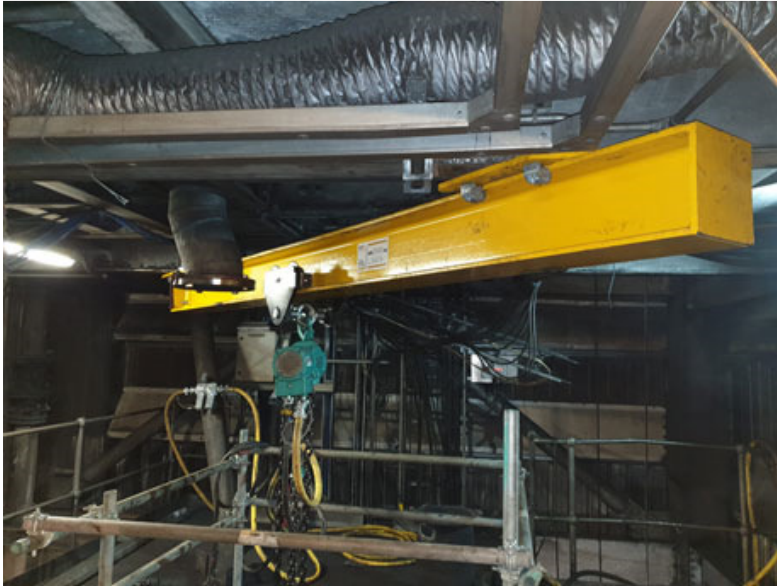
A strong Hoist and Winch business area is hoist hire, including higher capacity air/electric hoists, shown here a 5t air hoist.
