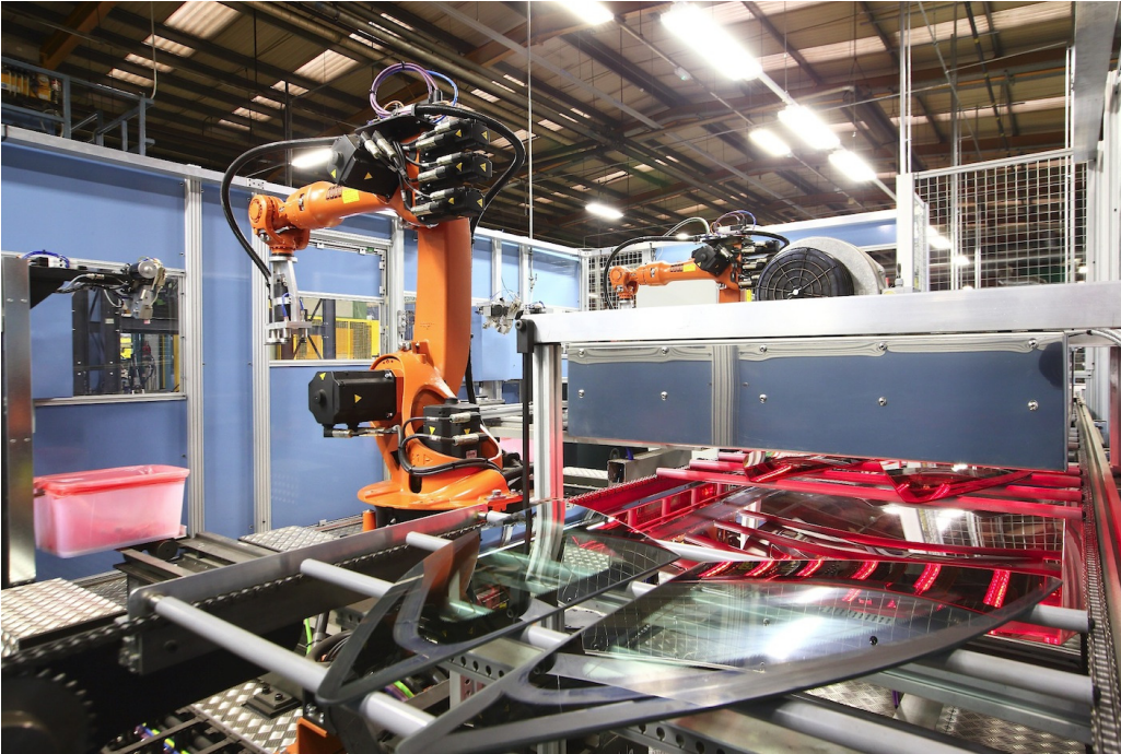
The Heraeus infra-red heating system in the robotic cell at Dura Automotive.
