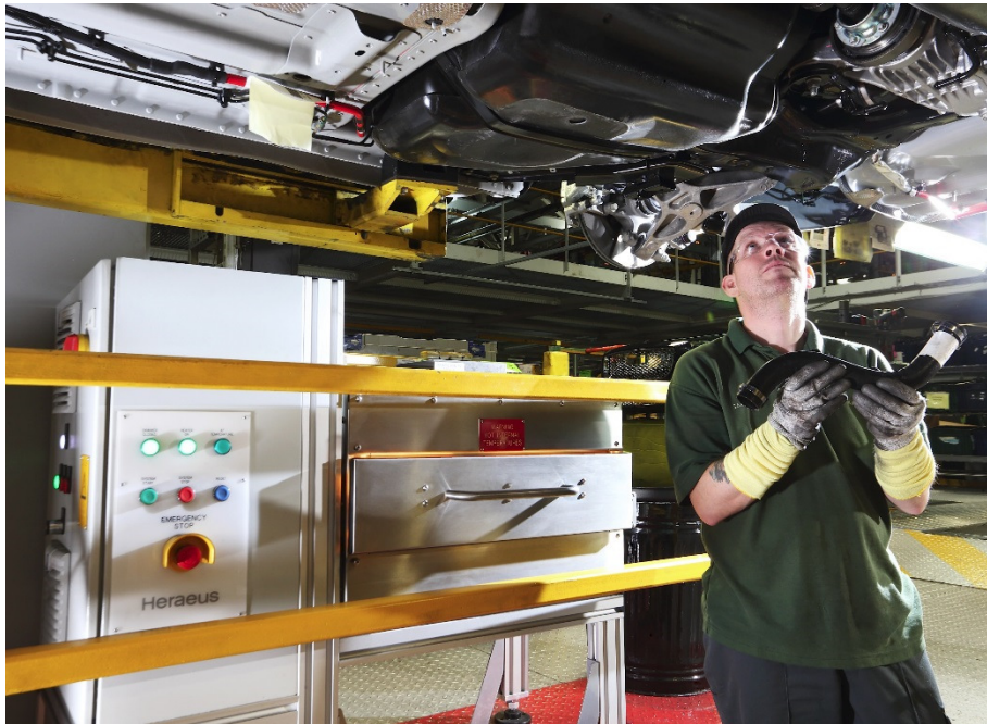
The Heraeus oven for softening fuel pipes before fitting at Jaguar Land Rover
