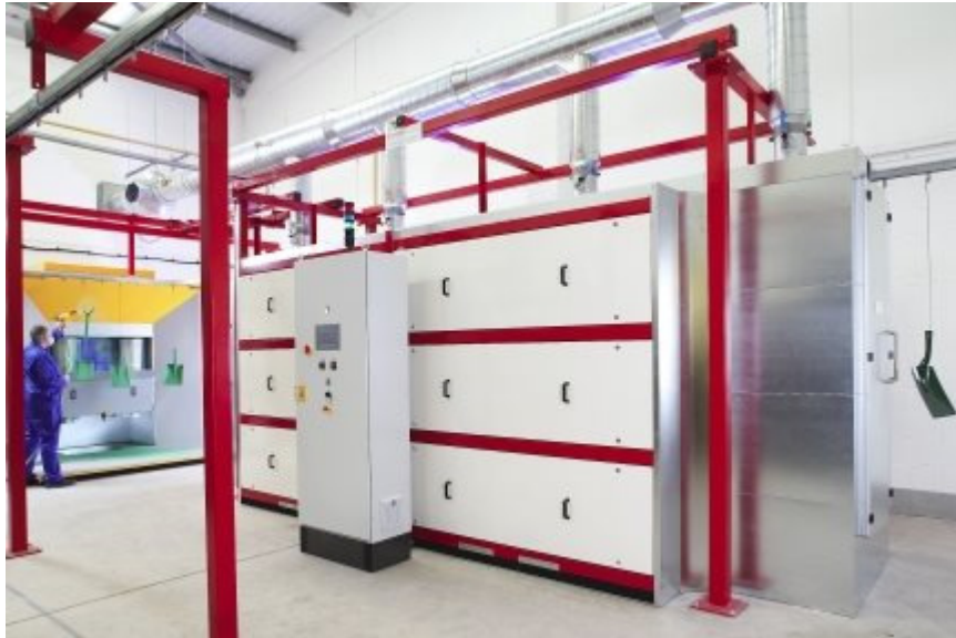
The Gas Catalytic IR oven at Heraeus
