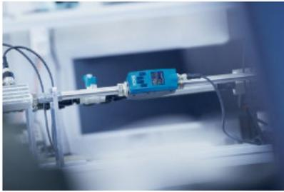
The SICK FTMg flow sensor measures flow, pressure and temperature simultaneously
