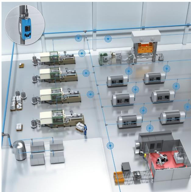
The SICK FTMg flow sensor can be positioned to identify leaks based on pressure losses, thereby minimising the operating costs for producing, supplying and distributing compressed air.
