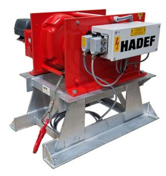
Control of the winch is via a low-voltage radio remote with back-up plug-in pendant. Features of note include: a pressure roller for the wire rope drum; four-position top/bottom geared limit switches; a galvanised steel mounting frame for the winch; and electrical enclosures with IP66 protection rating.
