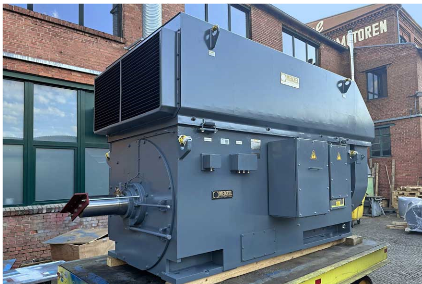
Caption: Menzel's large warehouse and modular design for motors and coolers allow fast delivery of tailored motor systems for industrial applications (here: 2000kW 11kV cement mill motor)
