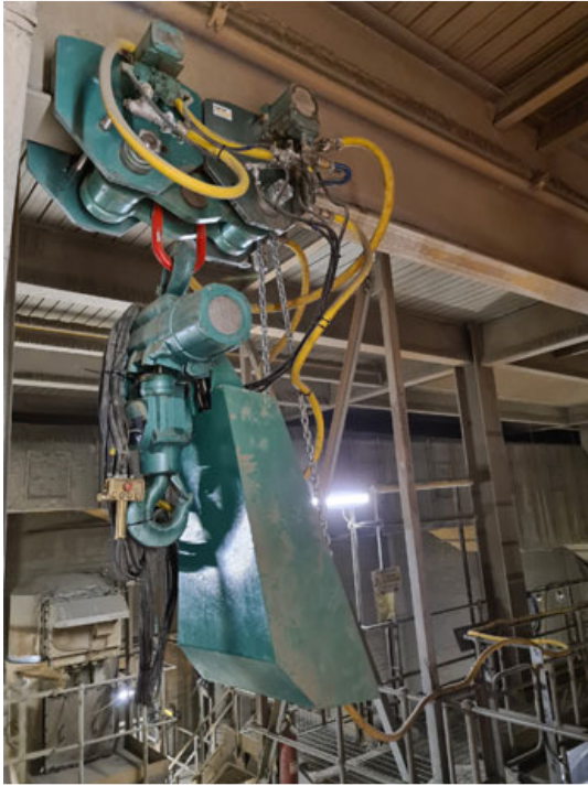
Special twin trolley 12t swl JDN air powered hoist.
