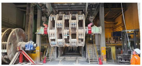
With a total weight of 80T, rotor lifting was courtesy of a pair of tandem-controlled 41T SWL wire rope hoists located on monorail beams arranged at  $90^{\circ}$  to the rotor bearing journal stub shafts.
