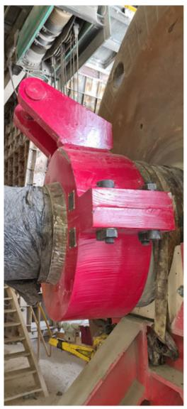
Hoist & Winch designed and manufactured two 41T SWL rotor lifting lugs to assist the lifting process.
