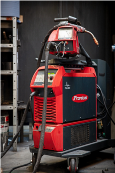
Figure 7: The welding machine with which Guntamatic has renewed the manual welding sector: The Fronius TransSteel 4000 Pulse.
