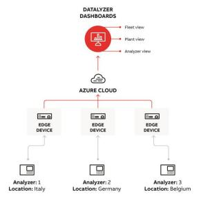
Datalyzer collects data from emissions monitoring analysers across the business which is then routed to an on-site Edge device that sends the relevant information to the Microsoft Azure cloud.
