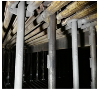
Fig. 8 – single tube #31 sprayed with IGS B450; #33 sprayed with IGS S475
