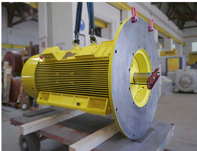
Caption: Menzel had a suitable motor in stock and made all necessary modifications for this pump application within a short time, including a special oversized flange for vertical mounting
