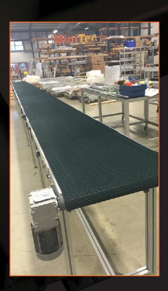
The height adjustable guide rails were also manufactured to be well-equipped to cope with the demanding production requirements and variety of parts which will pass over them.
