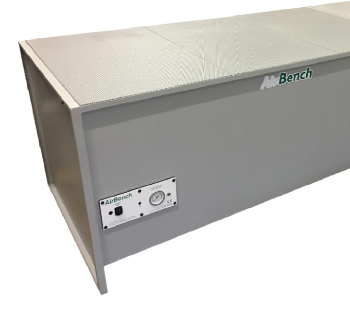
AirBench FPW is designed for production level welding and grinding, generally on mild steel and similar materials. Both sizes use energy efficient EC fans and run from a standard 13a single phase supply. Grinding dust or weld fume is drawn downwards through the ventilated surface and filtered, before clean air is returned to the room. As with all standard AirBenches, no installation is required.
