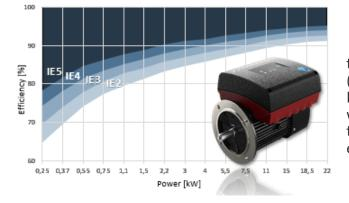
"the losses in an IE5 motor is more than 30% lower than the IE3, this alone reduces the energy consumption by **10%** with a typical pump profile"
