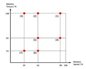
measurements of losses at seven standardized load points as foundation for the EEI calculations.
