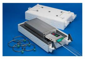
**Illustration:** The quick-cool-down, no-outgassing system enables frequent profiling of product temperatures even during normal production
