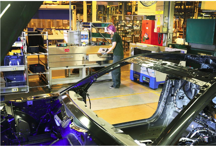
The Heraeus IR oven on the production line fitting sound-deadening pads to the Jaguar F-TYPE at Jaguar Land Rover's manufacturing site at Castle Bromwich
