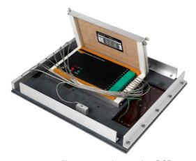
**Illustration:** The temperature profilers are used to monitor PCB temperatures and oven performance – via sensor fixtures like this one
