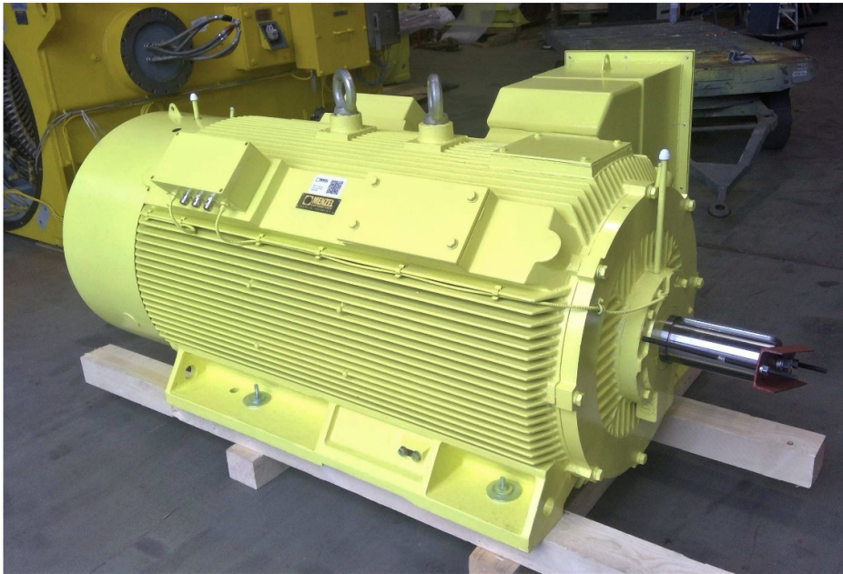
Frame MEBKGR355-04 600HP 3300Volts 1500rpm Sewage Aerator Drive
