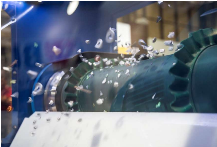
Figure 2 - Dynamic separation of non-ferrous metals on the Eddy Current Separator
