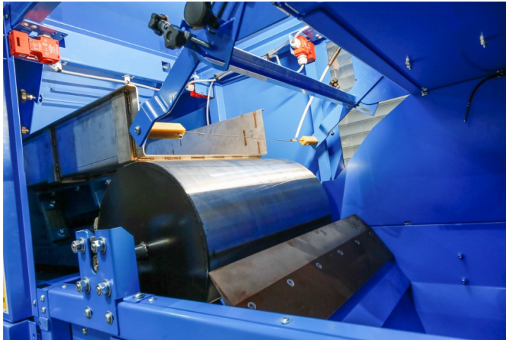
Figure 1 - Inside the ElectroStatic Separator
