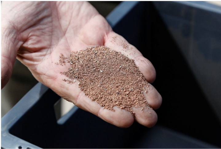
Figure 5 - Recovered fine copper wire at 95% purity
