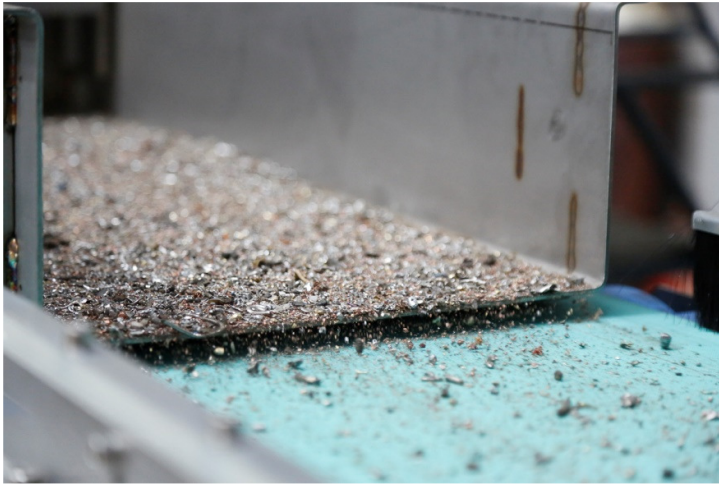
Figure 2 - Metal mix feeding onto the second stage Rare Earth Roll Separator
