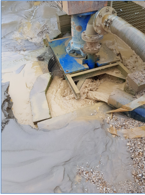
Caption: Aggregate production demands a high volume of water which returns to a sump for pumping to a settling bed
