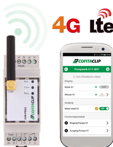
Illustration: The configurable communication modules enable remote control and maintenance via 4G wireless networks
