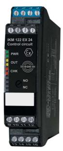
**Illustration:** The IECEx-certified signal processing unit for installation outside gas and dust explosion hazard zones connects to intrinsically safe two-wire sensors
